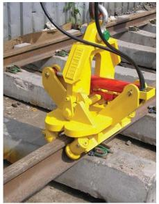
Max. Hyd Pressure 210Bar Min. Hyd Pressure 90 Bar Body Colour 08E51 Yellow Cylinder colour Signal Red
